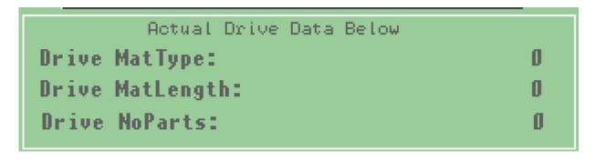
If the EP-P is connected and the tags are configured correctly then when you press the send drive button the data should display on the Actual Drive Data section.
